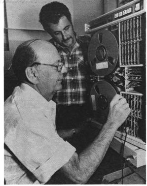
JIM HAWKINS (foreground) and Keith Vollmer analyze data tapes from joint-interface lab tests — systems tests done elsewhere. Joint-interface tests check out Sandia-designed DOE packages and military adaption kits
